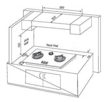
\*To combustible surface (dimension is not relevant if the adjacent surface is non-combustible).
