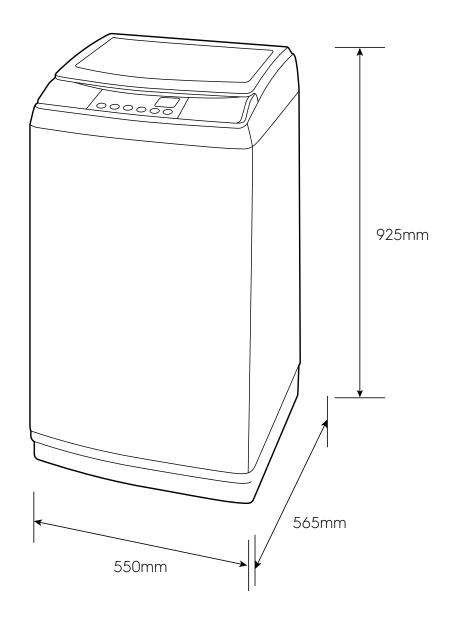
Please note! Dimensions to be used as a guide only. All customers MUST refer to the user manual supplied with the product for detailed installation instructions. © 2021 Electrolux S.E.A PTE. LTD. E\_DIM\_EWT8588H1WB\_Aug20
