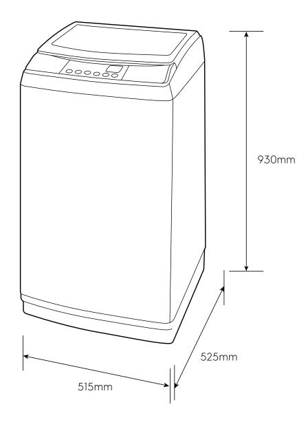
Please note! Dimensions to be used as a guide only. All customers MUST refer to the user manual supplied with the product for detailed installation instructions. © 2021 Electrolux S.E.A PTE. LTD. E\_DIM\_EWT7588HIWB\_Aug20
