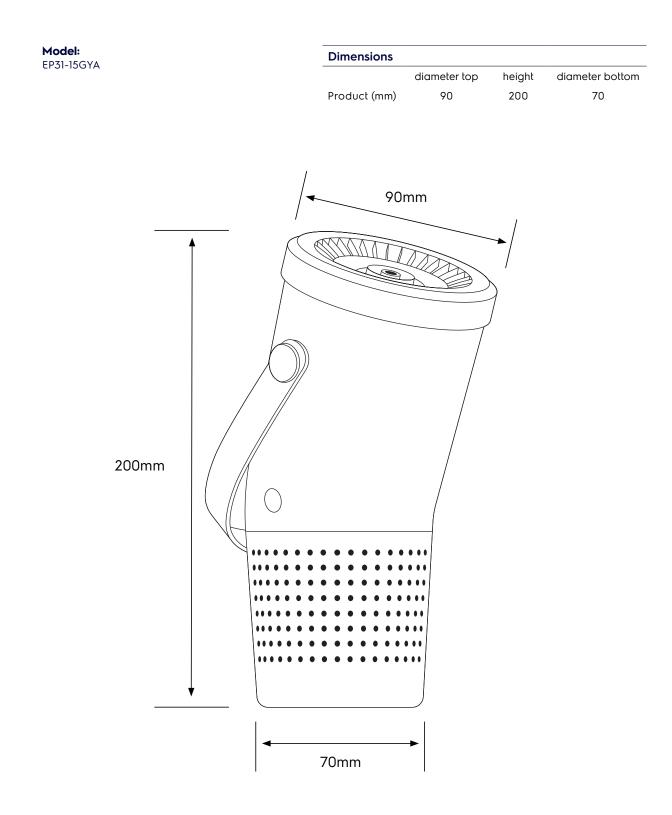
Please note! Dimensions to be used as a guide only. All customers MUST refer to the user manual supplied with the product for detailed installation instructions. © 2021 Electrolux S.E.A PTE. LTD. E\_DIM\_EP31-15GYA\_Nov21
