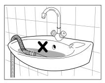
In a sink, drain pipe branch.
