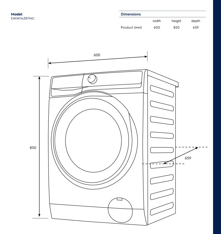
Please note! Dimensions to be used as a guide only. All customers MUST refer to the user manual supplied with the product for detailed installation instructions. © 2024 Electrolux S.E.A PTE. LTD. ELX\_DIM\_EWW1143R7MC\_ID\_Mar24
