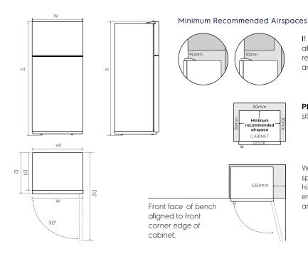
If you do not have a cupboard with allowance for air flow above the refrigerator, the recommended clearance
