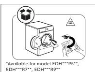
For model **EDH\*\*\*J5\*\***, Use the DRUM UNLOCKED KEY to unlock Rear Drum locks, before using the appliance. For other models, the rear drum locks are removed automatically when the dryer is activated for the first time. Possible to hear some noise.
